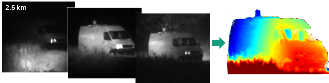
Figure 7: Sliding gates sequence and resulting range image of a vehicle at a distance of 2.6 km.
