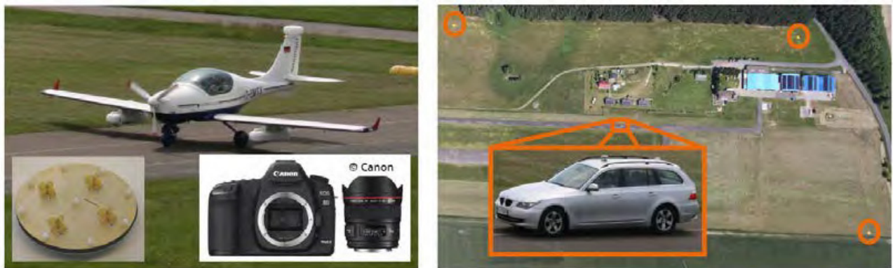
Figure 9: Experimental set-up for a measurement campaign involving emitter localization (DoA) and optical sensors: aerial platform (manned UAS demonstrator), 3 stationary, 1 moving object to be localized.
