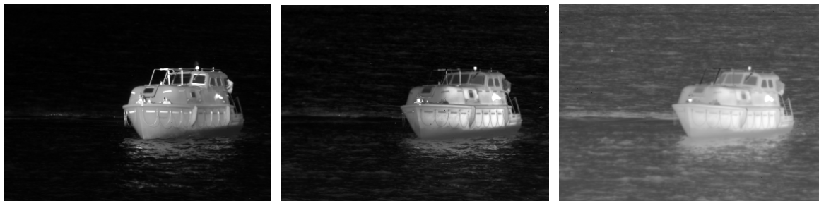
Figure 2: Infrared images of a boat in different wavelength ranges. Left: short-wave IR 1.2-5 \mu\text{m} . Middle: mid-wave IR 3-5 \mu\text{m} . Right: long-wave IR 8-9 \mu\text{m} (from [11])
