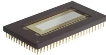
Figure 8: 1 MPixel SLM chip
