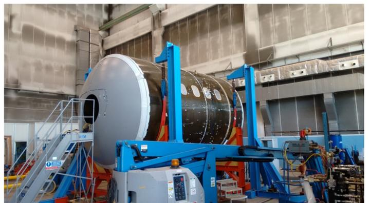
Figure 1: Ground test in the laboratory: A special measurement setup detects the cyclic internal pressure load on an aircraft fuselage simulated by inflation. Photo: Leonardo
