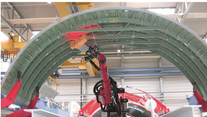
Ill. 1: Fuselage section assembly inspection system (Fraunhofer IFF)
