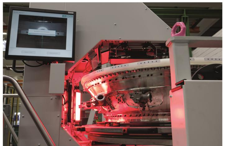
**Ill. 4: Assistant for TCF module assembly inspection (Fraunhofer IFF).**
