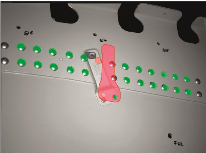
III. 6: Inspection and test result: faulty assembly (Fraunhofer IFF).
