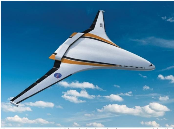
Figure 5: NASA N3-X blended wing body concept with distributed turbo-electric propulsion [9]
