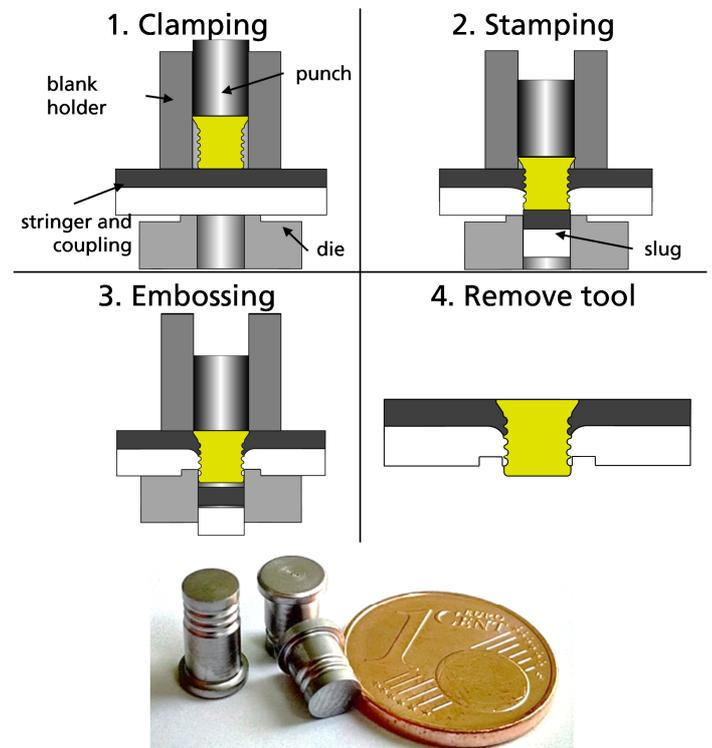
Figure 2: Process steps for a SPR joint (top) and SPRs in comparison to 1 €-cent
