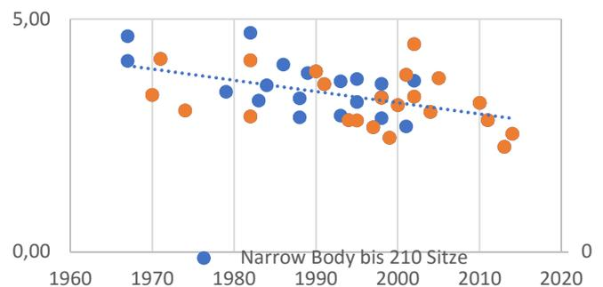
Figure 1: Fuel consumption per passenger (left axis l/100 km, right axis CO<sub>2</sub> emissions kg/100 km) Calculations based on European Emission Agency (2016) [6], [7]
