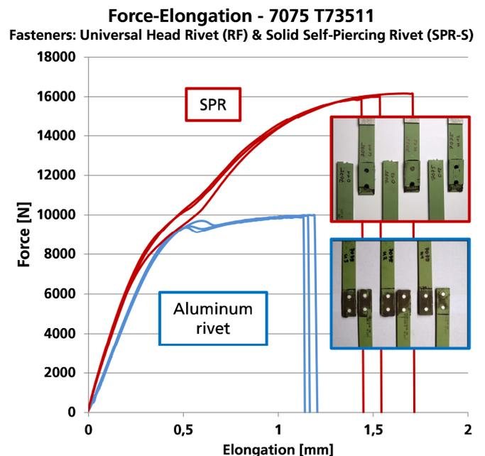
Figure 3: Shear strength of conventional  $\varnothing$  4,8 mm aluminum rivet compared to  $\varnothing$  4,0 mm steel SPR
