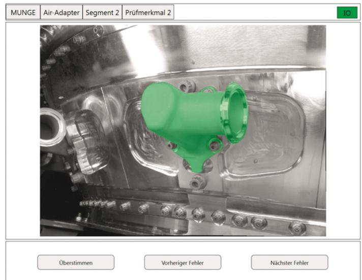
Ill. 2: Inspection and test result: attached part and joints correct, some missing joints and missing boreholes (Fraunhofer IFF)
