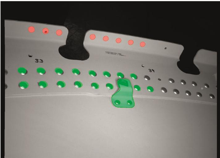
III. 5: inspection and test result: correct assembly (Fraunhofer IFF)
