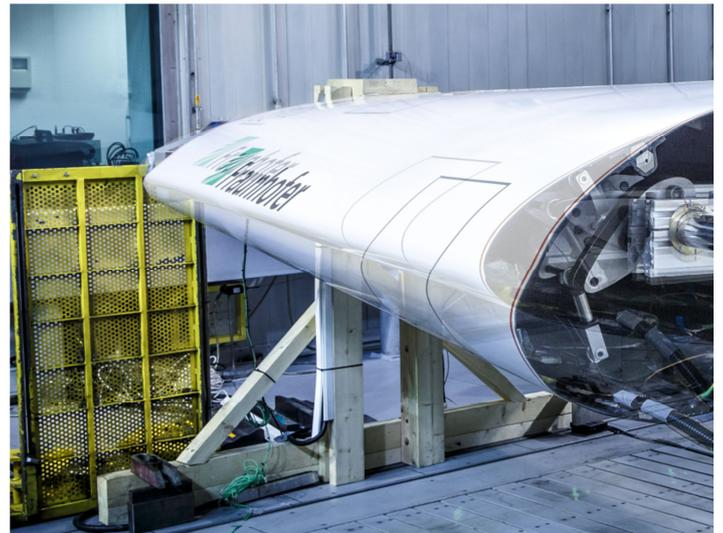
**Figure 1: Wing structure with flexible droop nose.**
