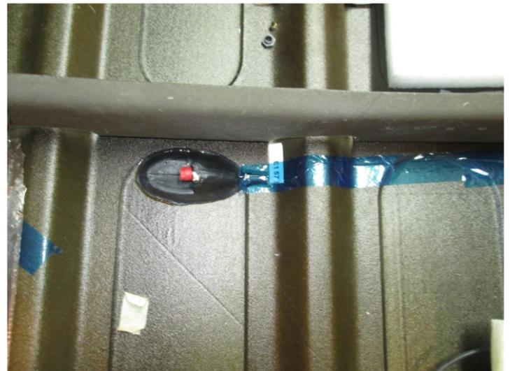
Figure 3: Fraunhofer LBF connector hub for integrated sensors in composite structures.
