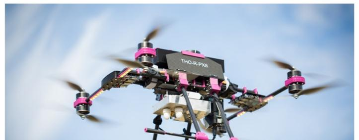
Figure 1: With the ACoRad-94 on an octocopter, flight altitudes and distances can be measured down to the last centimeter at any time.
