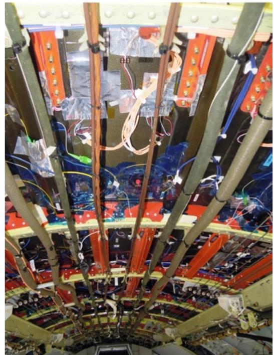
Figure 3: Optical sensors illustrate the deformation of the carbon fiber aircraft structure very accurately. Photo Fraunhofer LBF
