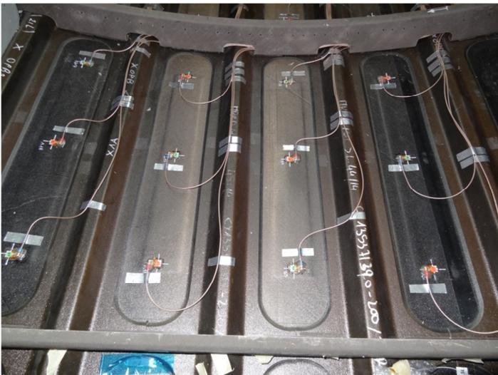
Figure 2: The high-precision measurement setup from Fraunhofer LBF can detect and display the deformations to carbon fiber structures very accurately
