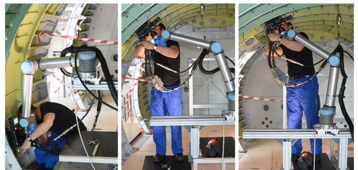
Figure 1: Riveting using human-robot collaboration
