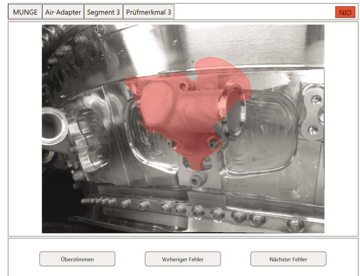
Ill. 3: Inspection and test result: skewed attached part, correct joints (Fraunhofer IFF)
