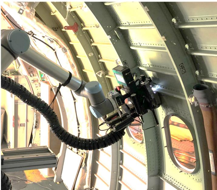
Figure 5: Installation tool at trials in an old airplane
