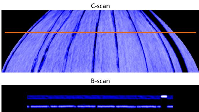
Figure 5: The C-scan shows the backside wall of a radome test structure, which is composed of several glass-fiber reinforced plastic panels. The orange marker indicates the position of the B-scan image below. The strong feature in the upper right of the B-scan comes from a metal stripe attached to the test sample, which completely reflects the measurement signal.
