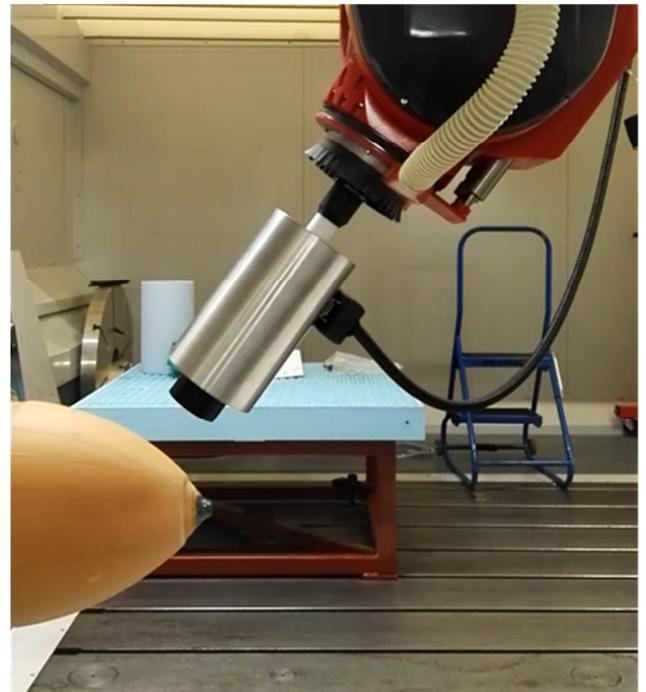
**Figure 4:** Terahertz inspection of a small radome test structure with the sensor attached to the tool holder of a machining center for radome manufacturing.
