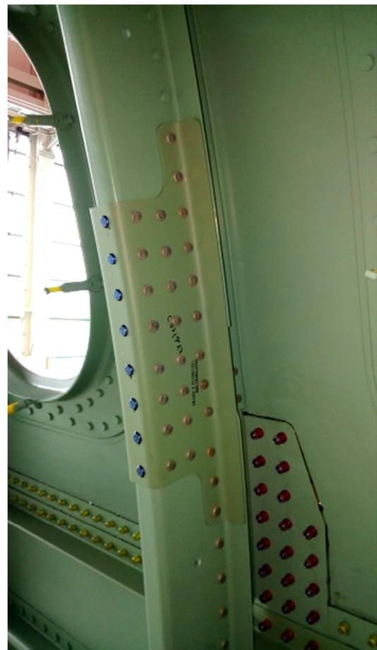
Figure 6: Frame coupling with conventional aluminum rivets
