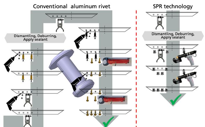
Figure 4: Comparison of the assembly processes
