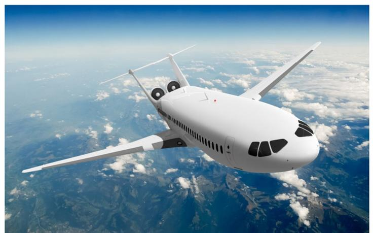
**Figure 3: D8 Double bubble concept with boundary layer ingestion turbofans [10]**
