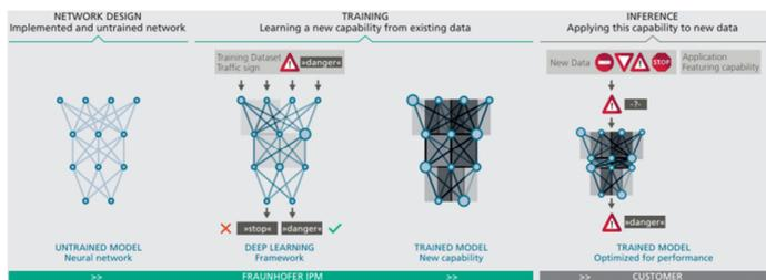
Figure 1: Process chain in a Fraunhofer IPM deep learning framework: Network design, training and application
