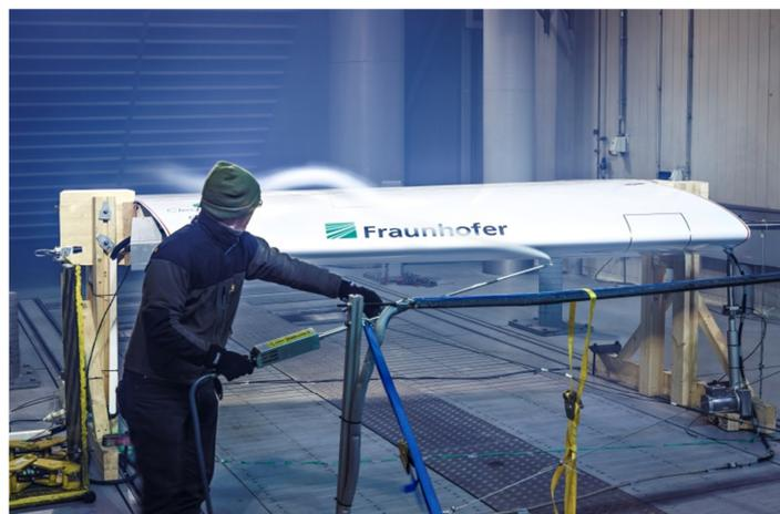
Figure 2: Use of a smoke lance in the climatic wind tunnel.
