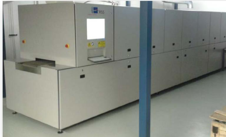
Thermal (IR or convection; air or nitrogen, 2400 wafers / h, manufactured 2015 by REHM, Germany)
