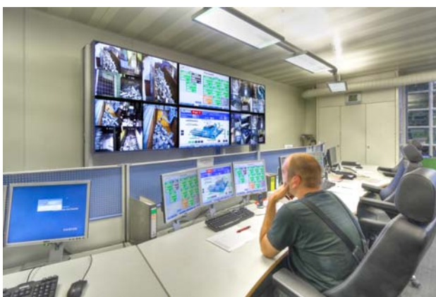
Figure 6 – Control room in a press shop – the entire factory on a glance (source: Jungmann Systemtechnik/Daimler)
