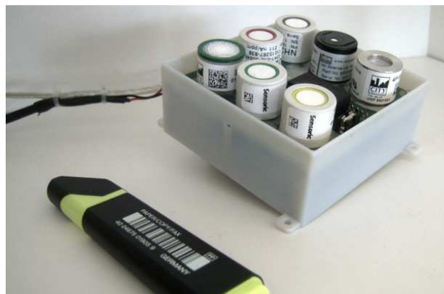
Figure 5. Gas sensor to detect inflammable gases, Ammonia, Nitrogen Dioxide, Sulphur Dioxide, Carbon Monoxide and Chlorine
